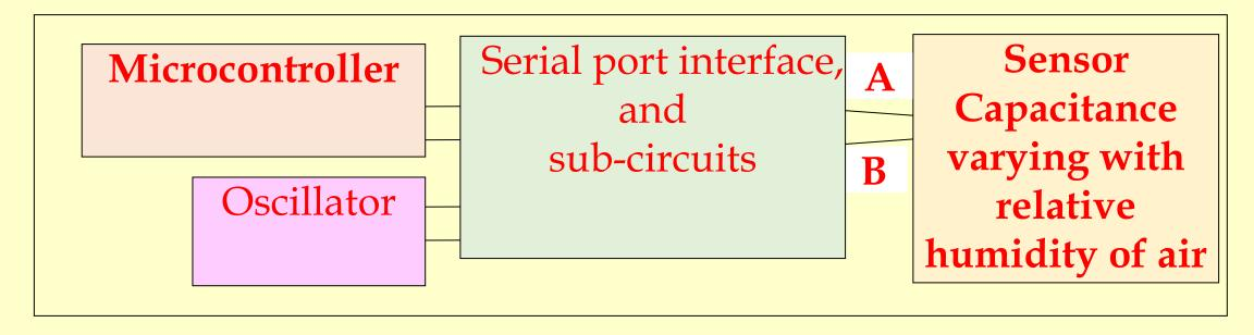
The microcontroller electronic-circuit port connected to interface and sub-circuits; and receiving input from a capacitive sensor whose capacitance value is varying with the relative humidity of air and the circuit sensing the variation in relative humidity
