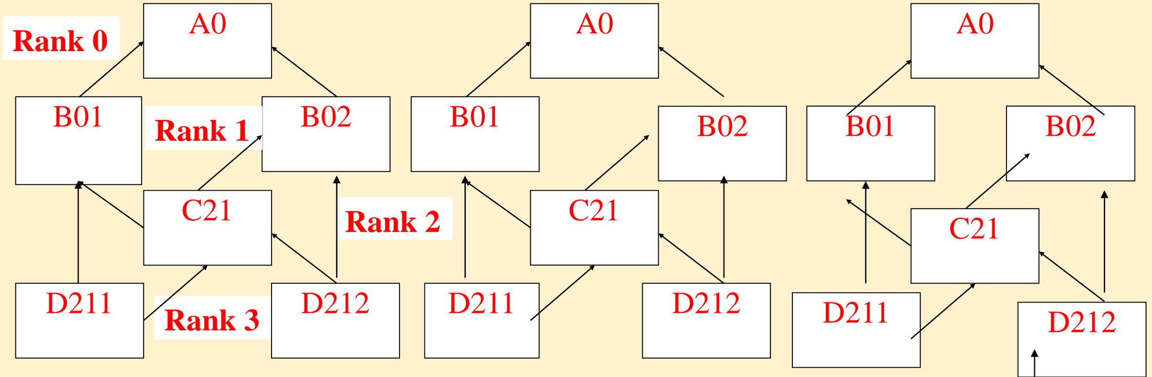
Fig. 4.4 RPL network nodes at four ranks and RPL data-flow instances for upwards and downwards flow
